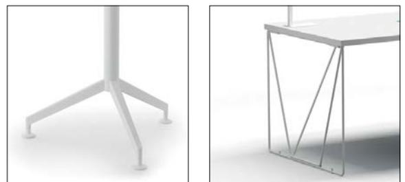
**DESK WITH TRESTLE LEG:** Fixed structure is made of calibrated rods of  $\varnothing$  11mm and covered with epoxy paint of 80 microns thickness. The structure, with a rectangular frame form, incorporates a supportive tight that gives support to the desk top.
