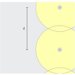
Castor bollard luminaires with 180° wide light distribution (h ≥ 800 mm) enable uniform path lighting with luminaire spacings (d) of up to 8m. Other distances can be selected to support optical guidance.
